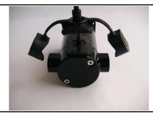
Slide the motor cord through the rubber cover and ensure that it is in the correct orientation. Remove the backing from the foam gasket.
