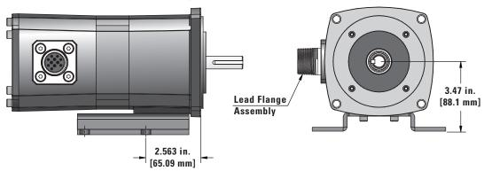
Type 34B6BXBL-FX BLDC or 34R6BXPP-FX Inverter-Duty Gearmotor with Base Mount Kit Installed
