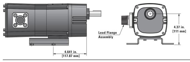
Model 0931 Base mount Kit Dimensions (Top dimensions are in inches. Dimensions in brackets are in mm)
