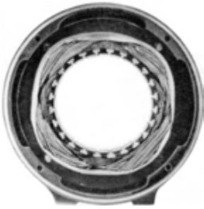
Fig. 2-11: Typical four-pole, split-phase stator.
