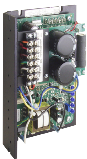
Filtered SCR Brushless DC Controls ABL Model 3911 & 3912 (enclosed); 3910 unfiltered SCR (130VDC)
